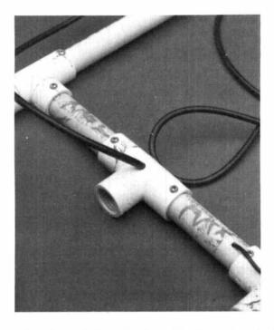
ens the wire and allows it to be cut to size and worked easily. A good grade of twin lead works well, and is easier to keep in place inside the pipe.
