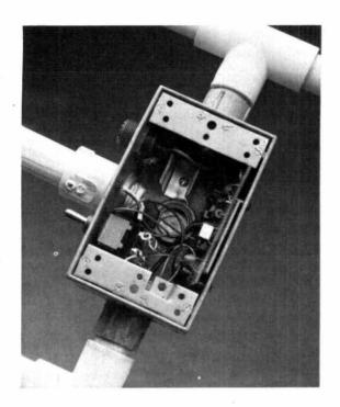
waterproof outlet box with five threaded 1/2-inch holes. Purchase a box at an electrical supply outlet; a Mulberry no. 30221 or equivalent is needed. This cast aluminum box with its waterproof cover can be used at the center of the array to house the electronics and perform the job of a tee section. Electrical and plumbing supply houses carry threaded to slip joint transitions. The electrical (gray) ones thread into boxes easily.
